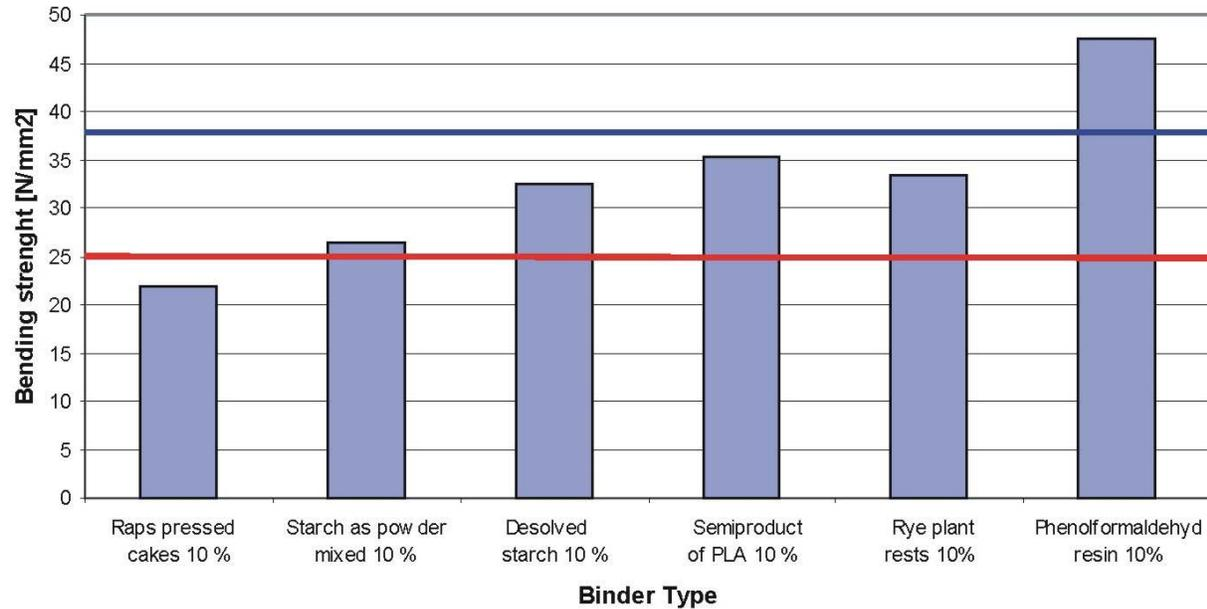
Fig. 6: The bending strength of natural fibreboard with different binders (material: hemp silage mixed with wooden fibre 6:4, density 1140 kg/m<sup>3</sup>, thickness 10mm). — minimum required strength towards EN 622-2 for HDF boards for common purposes in dry area, and — for highly reliable boards for construction purposes in moist area.
