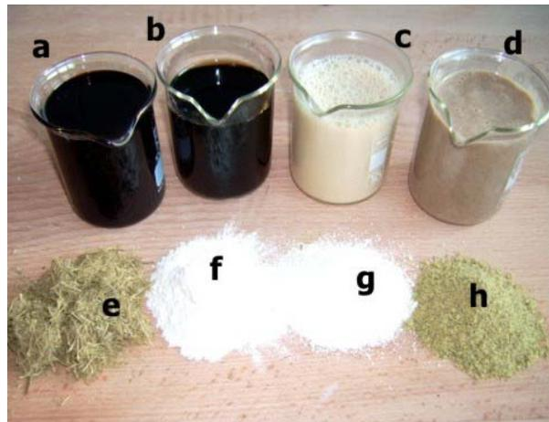
Fig. 4: Used materials: a-Phenol resin, b-PLA semi product, c, d-plants rests of glucose production, e-fibre, f-starch, g-cellulose, h-raps pressed cake
