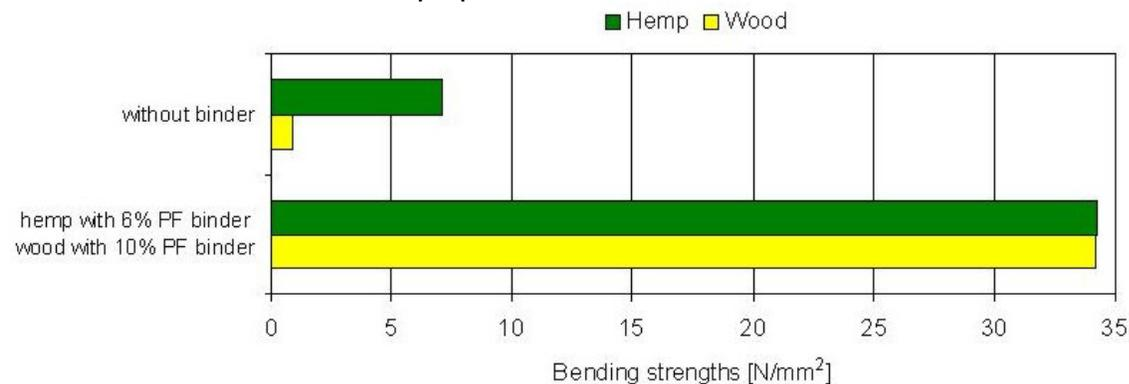
Fig. 7: The bending strength of fibreboard made of hemp and wood fibre (thickness 10 mm, density 790 kg/m<sup>3</sup>, pressing time 6 min., binder PF resin)
